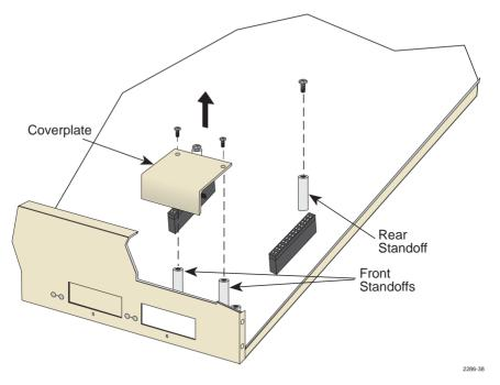
Figure C-4 Coverplate Removal
